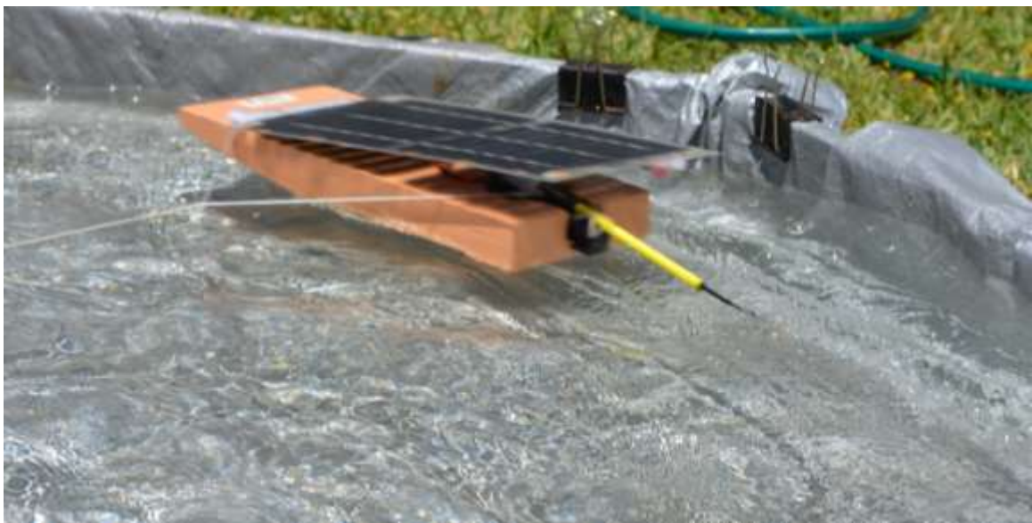
Test boat running at speed in a pool. (100% Sun race time expected is 3.9 seconds)
